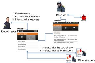
Figure 5: Rescue scenario: SW modules and main interactions.
